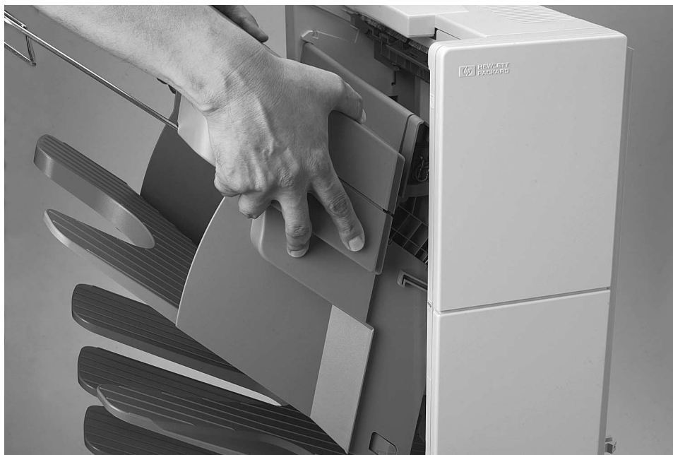
Figure 6-180 Mailbox with Stapler, Stapler Removal or Installation
