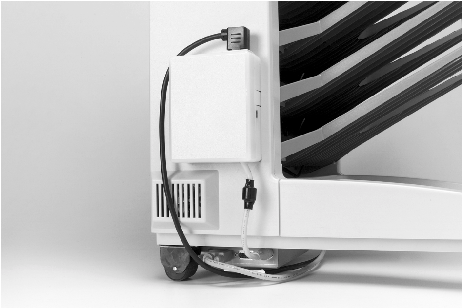
Figure 7-24 8-bin Mailbox Power Supply Test Mode Switch
