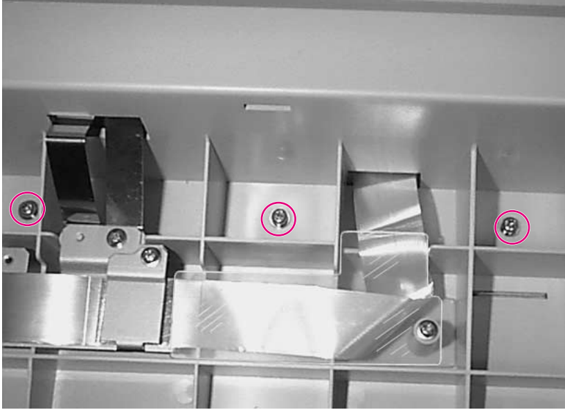
Figure 6-214 Front Panel Brackets (1 of 2)
